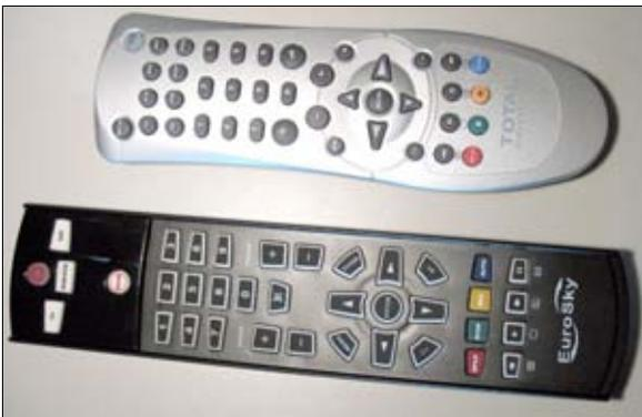
The IR receiver allows the RP6 to receive IR-signals from standard TV/Hifi remote controls, but this is restricted to remote controls using the RC5 code! Most of the universal remote controls (see fig.) may be programmed to this code – please read the manual of your remote control to set up the RC5 code. If RC5-code is missing in the code table, you may simply test several different manufacturers.
