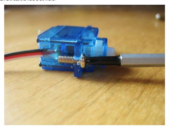
You can now easily fit your 25mm (1 inch) brass hex spacers. Use your pliers if necessary to hold the brass spacers when tightening the screws. **Do not over tighten** otherwise you will crack the servo mounts.
