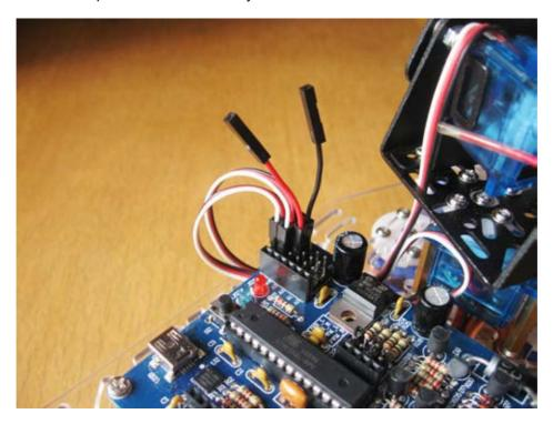
The motor control circuitry connects to the processor via 4 jumpers. Remove the jumpers on D8 and D10. Leave the jumpers on D7 and D9. This allows us to use D8 to control the IR LEDs on the eye. D10 might be used to control a small speaker or LED. The left motor control circuit is still connected and is used to drive a small shaker motor to make the tail wag.
