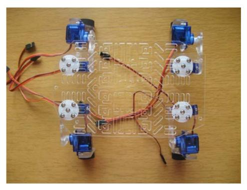
Step 8: Fit mounting spacers to pan servo.
